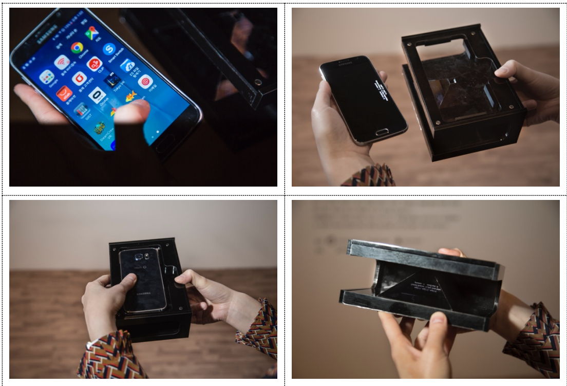
[Figure 25] A portable hologram device attached to a smartphone
