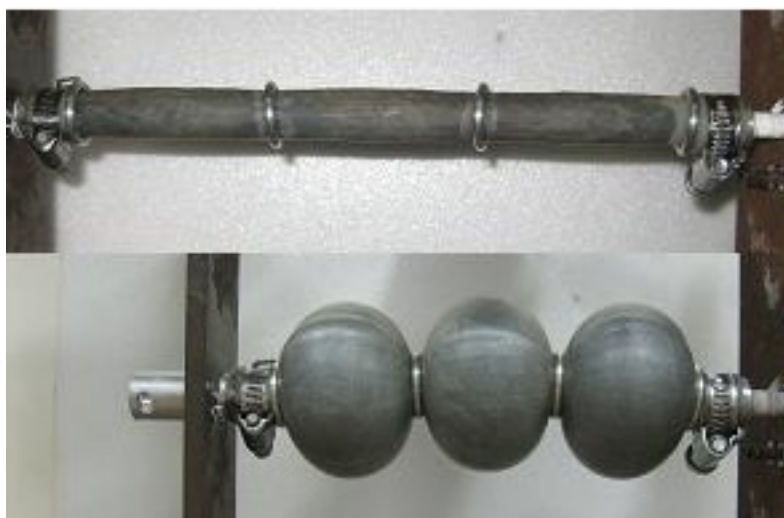
Fig. 2-4 Contraction of rubber artificial muscle with air pressure 11 .
