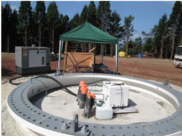
Fig.3 Wind resource measurement using LIDAR system
