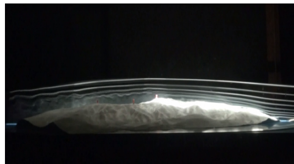
Fig.1 Wind tunnel test using actual topography model
