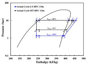
Fig. 1: P-h diagram of refrigeration cycles with suction gas superheating and liquid subcooling for HFC 134a for LT and MT; 4'-1 or d'-a: evaporation; 1-1' or a-a': suction superheating; and 1'-2" or a'-b": compression; 2"-3 or b"-c: condensation; 3-3' or c-c': liquid subcooling; 3'-4' or c'-d': expansion
