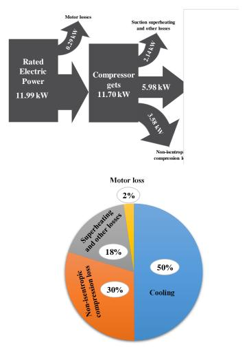
Fig. 4: Power distribution of a 27.7 kW (LT) compressor with HFC 134a refrigerant.
