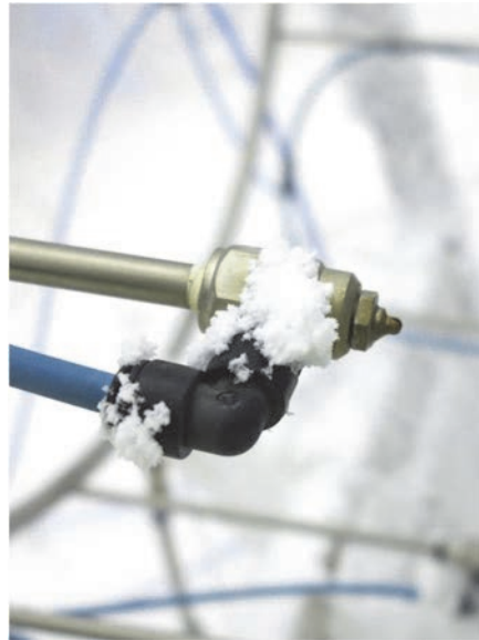
(b) Detail of single spray nozzle blowing into tunnel
