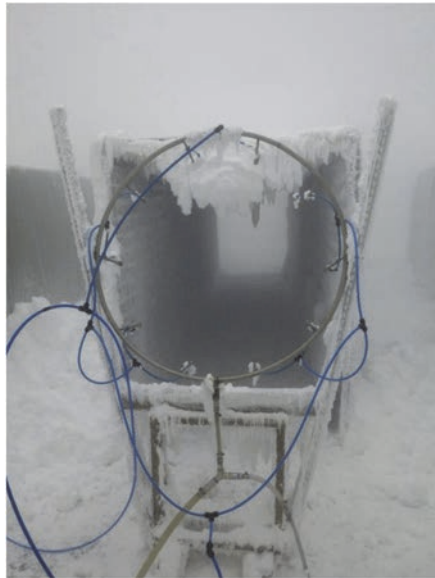
(a) Spray ramp with nozzles blowing into tunnel
