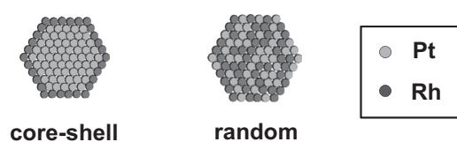
Figure 3 Cross sections of Pt-Rh bimetallic nanoparticle
