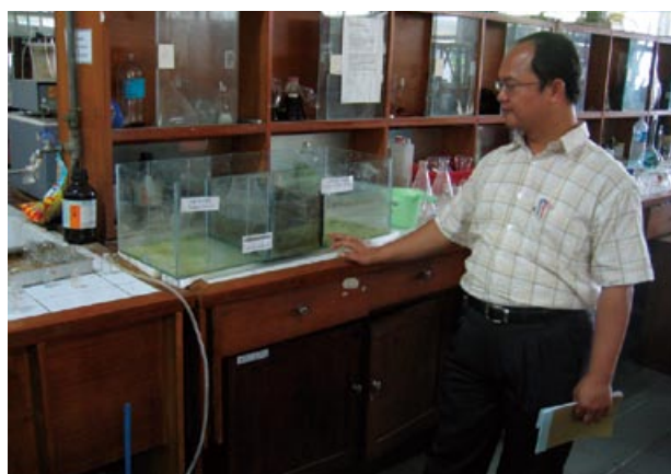
Fig. 2 Dr. Agus Prasetya of Chemical Engineering Department stands by his experimental apparatus for research on waste water treatment using bagasse.
