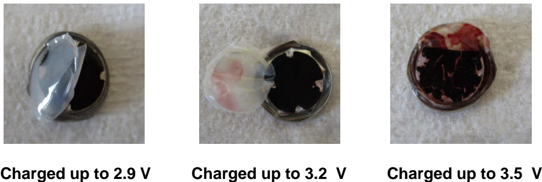
Figure 25. Pictures of electrode and electrolyte condition after charging to 2.9 V, 3.2 V, and 3.5 V.
