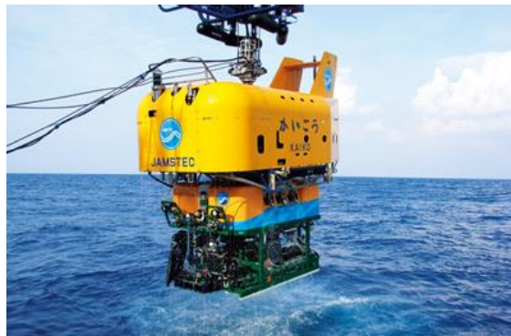
Fig. 1.1.2 “Kaiko 7000- II” which was developed to work in deep sea (JAMSTEC)
