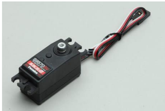
Fig. 2.7.1 Servo motor “S9570SV”
