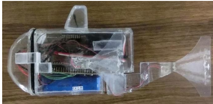
Fig. 2.5.5 Fish-type robot using artificial muscles and servo motor
