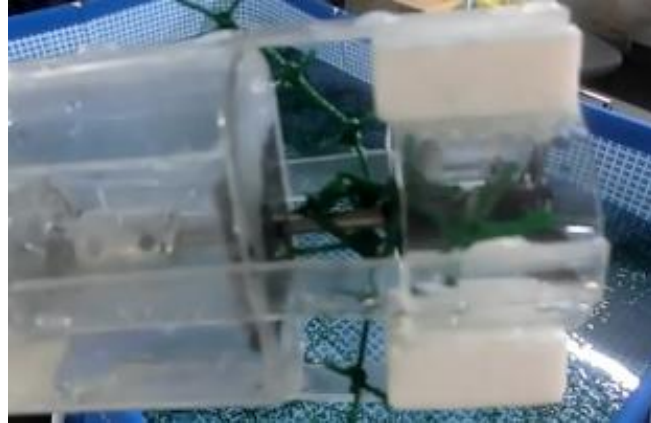
Fig. 3.7.4 Entangled imitation seaweed in thruster
