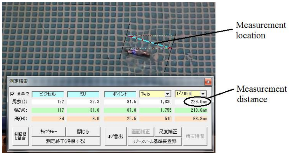
Fig. 2.6.2 Measurement of the position of swimming robot
