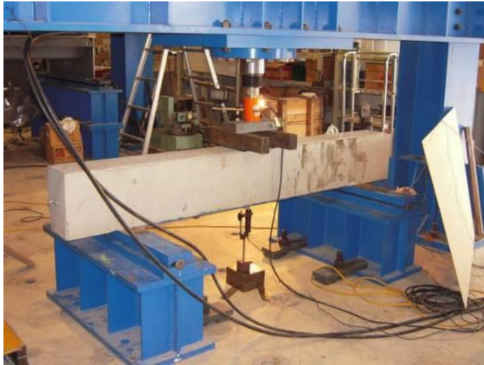
Photo 3.1 RC beam test
