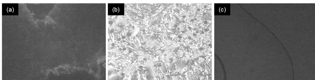
Figure 4-10 Polarised optical microscope images of the BBTME monomer: (a) 40 °C; (b) 220 °C; (c) 360 °C.
