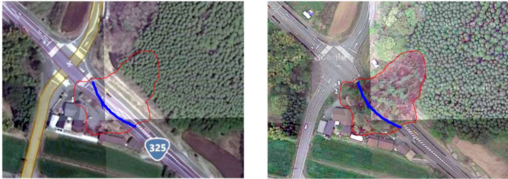
Figure 6-20 (a) Pre- and (b) Post-Earthquake image of the landslide case B. Red boundary shows the runout extent of the landslide. The blue line shows the landslide prone areas according to the Act on Sediment Disaster Countermeasures for Sediment Disaster Prone Areas
