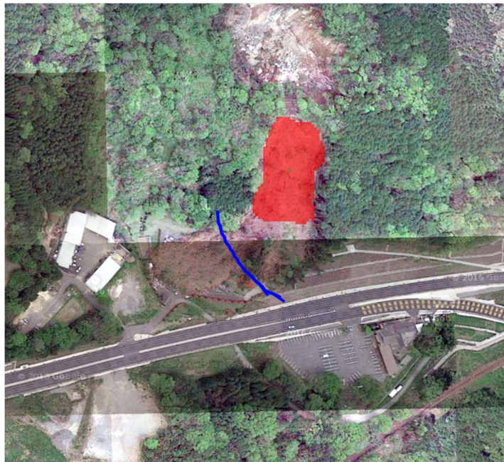
Figure 6-18 Landslide source area showing in red polygon
