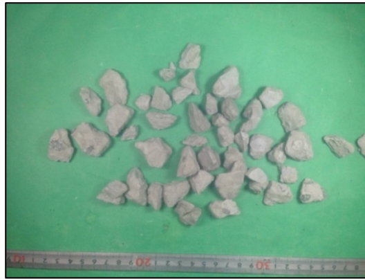
Photo 5.1 Covering reactive aggregates with cement paste w/c= 0.5
