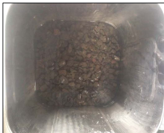
Photo 5.2 Reactive aggregates were immersed in LiOH·H 2 O solution
