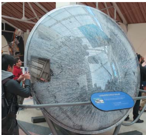
(a) Ablator on bottom surface of Gemini #11 (California Science Center)
