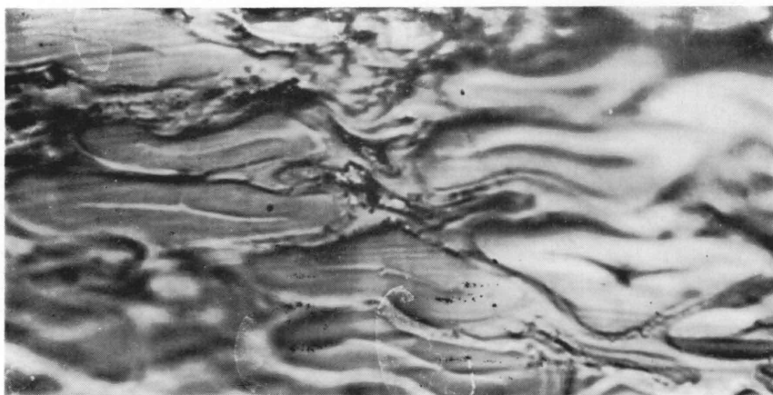
Photo. 6. Internal structure of fiberboard prepared from Asplund pulp of AKAMATSU wood, in the case of hot-pressing under 170^{\circ}\text{C} \cdot 80 \text{ kp/cm}^2 \cdot 20 \text{ min.}
