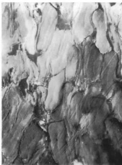
Photo. 5. Densification of internal structure of fiberboard hot-pressed at 170 °C for 20 min., with increasing pressure of hot-pressing.
