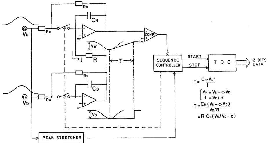
Fig. 2 Operational principle of the division circuit.
