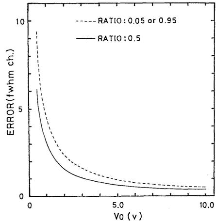
Fig. 8 Calculated errors as a function of the total pulse height value ( $V_0 = V_1 + V_2$ ) for various ratios ( $V_1/V_0$ ).
