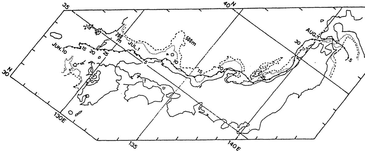
**Fig. 4** Trajectory of the surface drifter for the period from 6 June to 5 August, 1991 (after Ishii and Michida, 1996). Solid circles mark the location of the first fix of every day. Dotted and dashed line represent depth contour of 200m and 500m, respectively.
