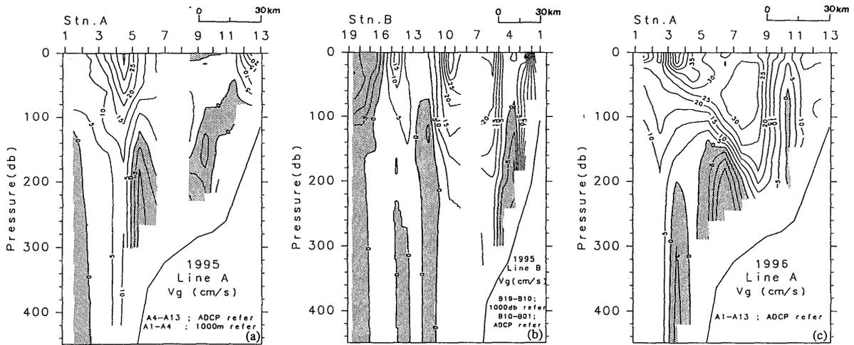
**Fig. 6** Vertical structure of the geostrophic current. The geostrophic calculations in 1995 from Stn. A4 to A13 and from Stn. B1 to B10 refer to the diurnally averaged current normal to each sections obtained by ship-mounted ADCP at the intermediate depth, while the calculations from Stn. A1 to A4 and from Stn. B10 to B19 refer to no motion level at the 1000m depth, and in 1996 refer to the diurnally averaged current by ship-mounted ADCP at the intermediate depth on the whole line.
