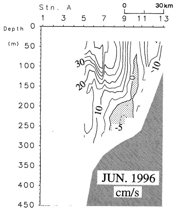
**Fig. 5** Vertical structure of the diurnally averaged current normal to the cross section of the line A obtained by the multi-level ADCP in 1996. Shaded area indicates the southwestward flow.
