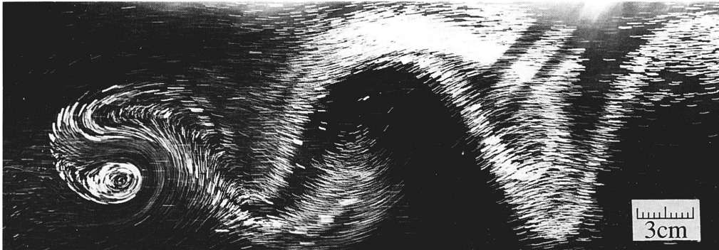
Fig. 6 Streakline pattern of periodic flow ( Q=7.29 , Re=375 , Rh=20.8 )
