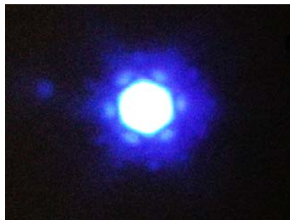
Fig. 2. Photograph of single mode fiber output. The image is saturated in the center region.
