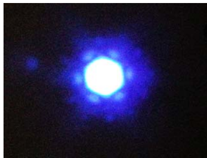
Fig. 2. Photograph of single mode fiber output. The image is saturated in the center region.
