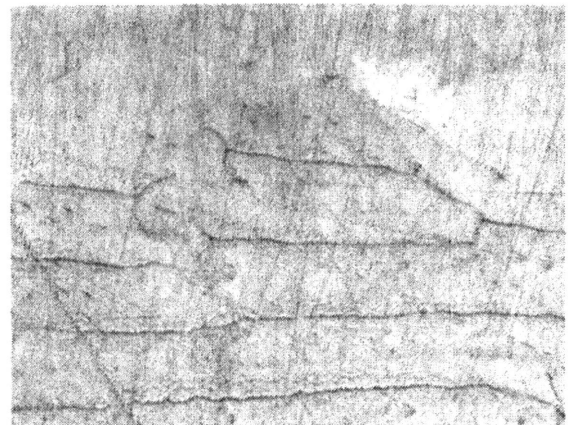
Fig. 7 Domain movement of 3% SiFe ( \times 200 ) (under magnetic field H= 1\text{ Oe} )
