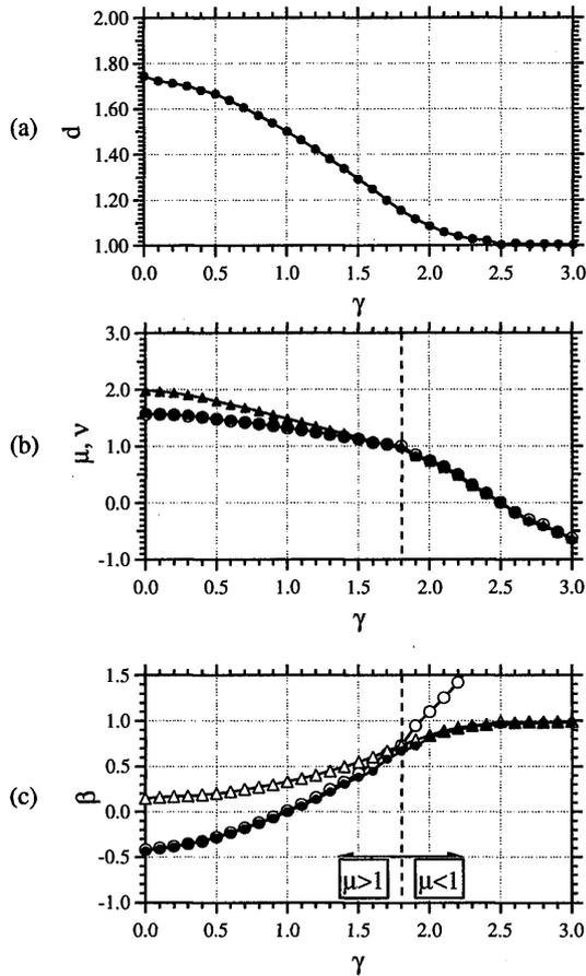
**Fig. 7** Dependence of several important indices to  $\gamma$ , the power law index of the magnetic field turbulence. (a) Fractal (capacity) dimension,  $d$  evaluated using Fig. 4, (b)  $\mu$  ( $\blacktriangle$ ) and  $\nu$  ( $\bullet$ ) evaluated using Fig. 5 and Fig. 6, respectively, and analytically estimated  $\nu$  ( $\circ$ ) by eq.(9), (c) diffusion scale index  $\beta$  evaluated numerically ( $\bullet$ ) and analytically ( $\circ, \triangle$ ) by eq.(20),(21).
