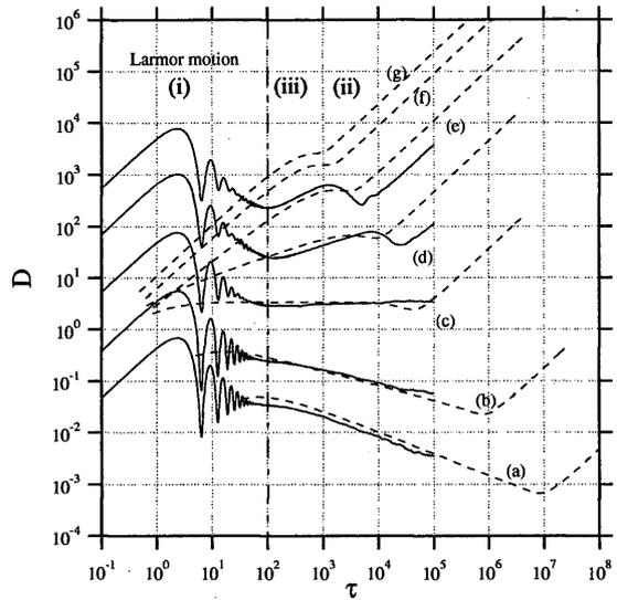
**Fig. 8** Time scale ( $\tau$ ) dependence of the diffusion coefficient ( $D$ ), which is evaluated by numerical integration of particle trajectories (solid lines) and by discussion of magnetic islands statistics (broken lines).
