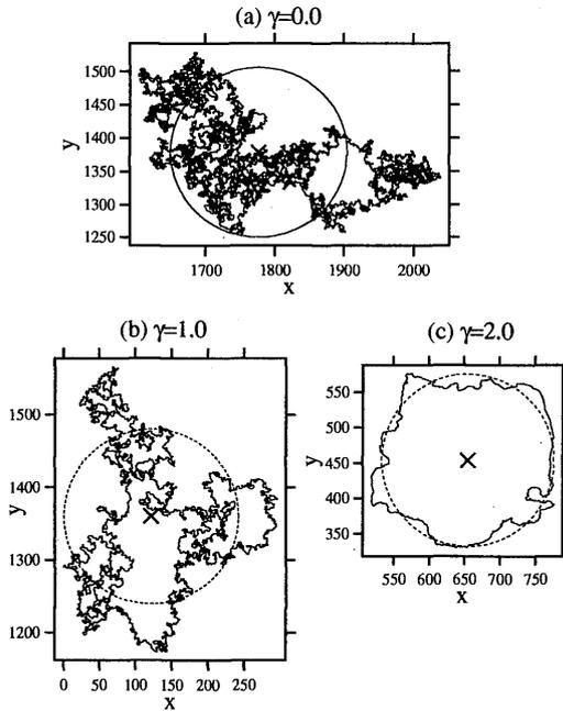
Fig. 3 Typical magnetic field islands for (a)  $\gamma = 0.0$ , (b)  $\gamma = 1.0$  and (c)  $\gamma = 2.0$ . In each panel, a circle is superposed with its radius ( $R$ ) evaluated by (5) and its center given by the gravity center of the trajectory.
