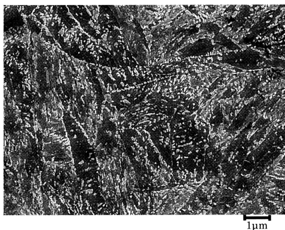
Fig.5(a) Martensite laths in JIS-SCM440 steel.
