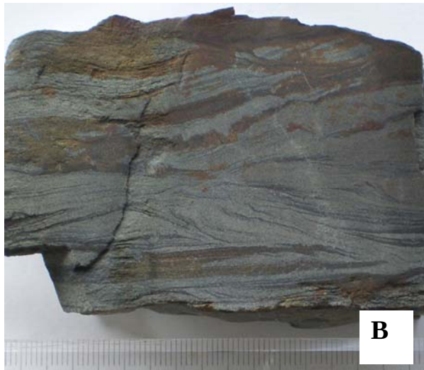
Fig.3.2.15 Outcrop photos show sedimentary features in sandstone on the southern coast of the Masuda. A: The alternation of thin sandstone and shale conformably overlies the thick sandstone bed (Fig.3.2.13). Climbing ripple cross-lamination and parallel-lamination which are reflected by decreasing and increasing flow velocity respectively. B: Wave-generated climbing cross-lamination (polished cross section of sandstone). C: Tererbellina preserved on the bottom surface of the thin sandstone bed. See the location and stratigraphic position in Figs.3.2.10 and 3.2.13, respectively.
