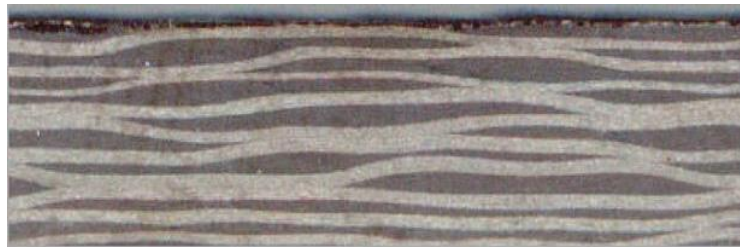
Fig. 4-1 Out-of-plane fiber waviness in a woven fabric laminate
