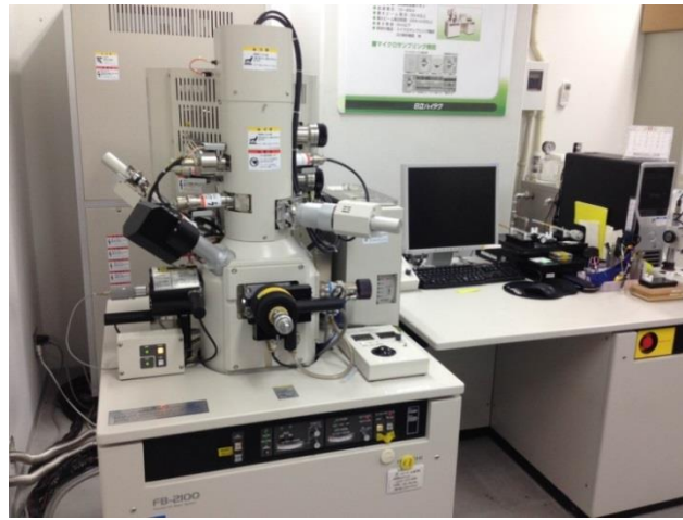
Figure 3-6. The FIB micromachining system (Hitachi High-Tech FB-2100).
