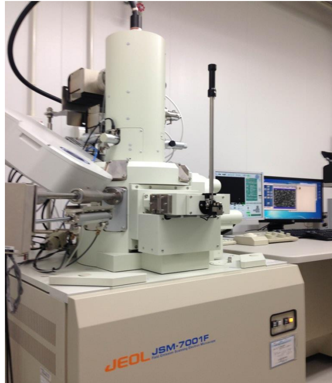
Figure 3-9. Field emission scanning electron microscope (FE-SEM).
