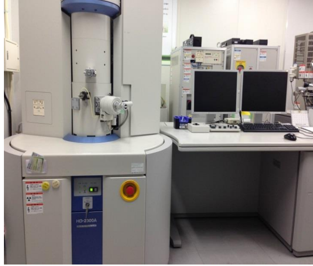
Figure 3-10. Scanning transmission electron microscope (STEM).
