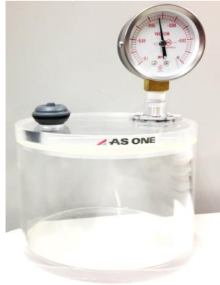
Figure 3-8. Desiccator for keeping samples in a vacuum.
