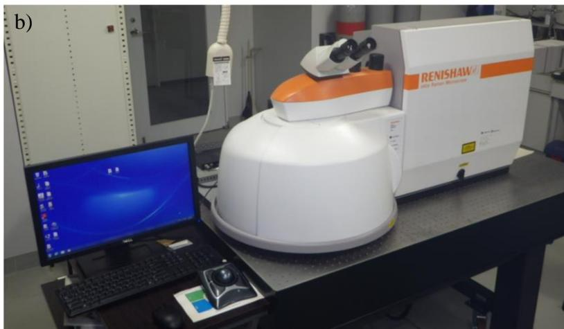
Figure 2.7. a) Principle of Raman spectroscopy. b) RENISHAW inVia Raman Microscope.
