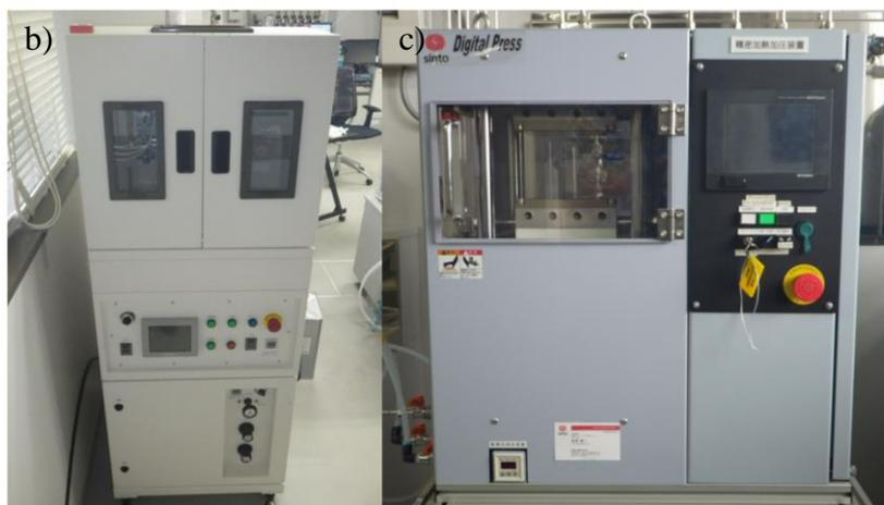
Figure 2.14. a) General fabrication process of a membrane electrode assembly. b) Nordson K.K. Spraying Device. c) Sinto Digital Press CYPT-10.
