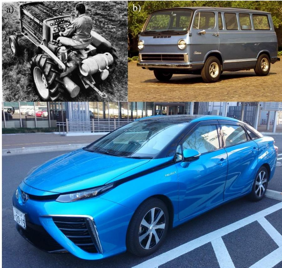
*Figure 1.2. Generations of fuel cell vehicles. a) The world’s first fuel cell powered vehicle, an Allis-Chalmers tractor with a 15 kW AFC stack, in 1959.<sup>26</sup> b) General Motor’s “Electrovan” with a 150 kW AFC stack, the world’s first fuel cell powered passenger car in 1967.<sup>28</sup> c) Toyota FCV MIRAI with 114 kW PEMFC stack, first commercial fuel cell vehicle in the world, in 2014.*
