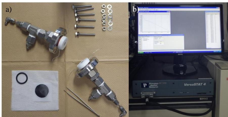
Figure 2.15. a) Cell holder used in our laboratory. b) Potentiostat VersaSTAT 4 (Amtek).
