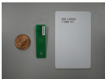
Fig. 2.7 RFID antenna and tag using in the robot.
