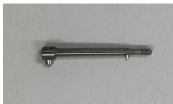
Fig.3.5 Appearance of contacting stylus
