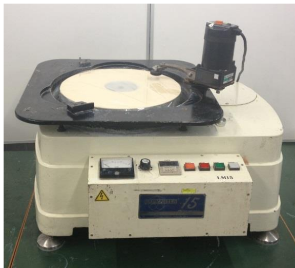
Fig.1.13. Exterior of polishing equipment LAPMASTER-15
