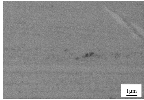
Fig.3.19 (b) Cross-scan irradiated substrate (1560s) after CMP
