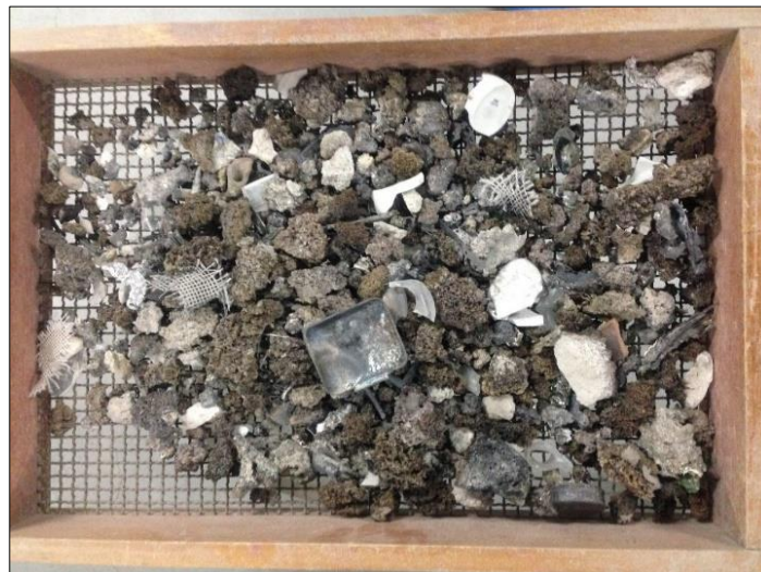
Figure 2.4 Grate siftings with particles larger than 4.75 mm obtained after sieving by mesh.
