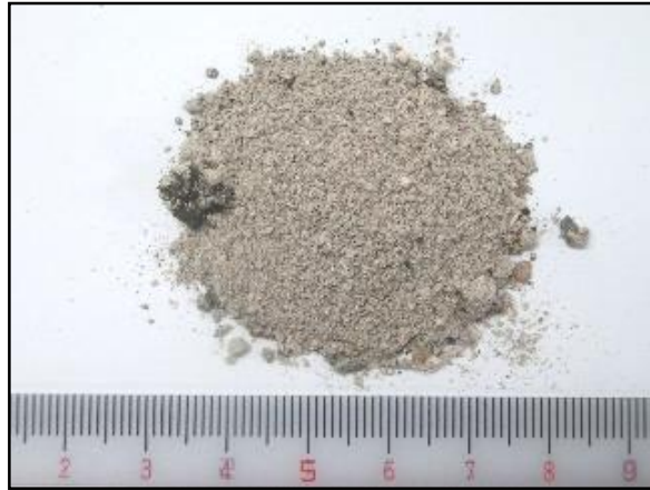
Figure 2.8 Physical appearance of unquenched bottom ash.
