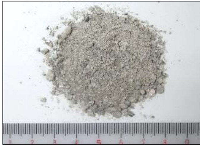
Figure 2.13 Physical appearance of the quenched bottom ash.
