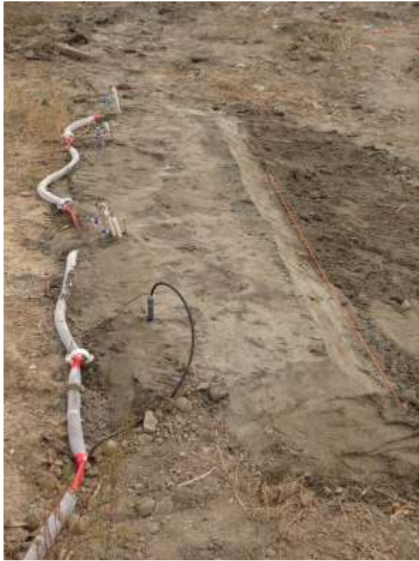
Final experimental set –up of the gas collection pipes
