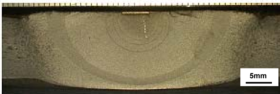
f) Peening, weld joint, \Delta\sigma_{R0.1}=200\rightarrow 220\text{MPa}
