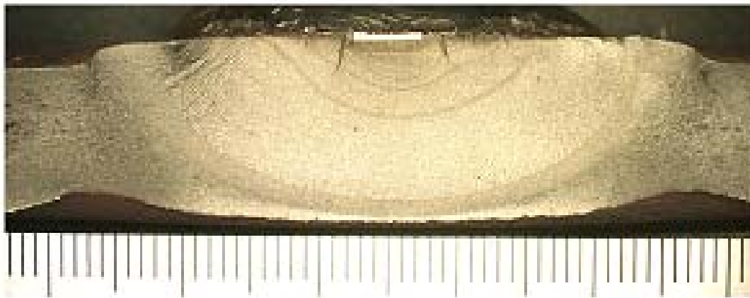
e) Peening, weld joint, \Delta\sigma_{R0.1}=220\text{MPa}
