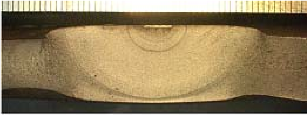
a) Non-peening, base metal, \Delta\sigma_{R0.1}=250\text{MPa}
