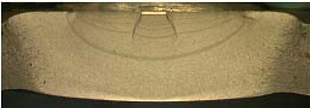
c) Non-peening, weld joint, \Delta\sigma_{R0.1}=200\text{MPa}
