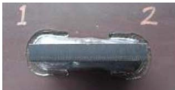
b) Hammer peening on base metal using square and flat pin
