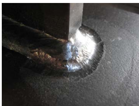
a) Hammer peening on base metal using 4.5mm radius semicylinder pin
