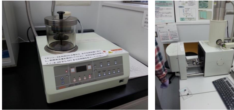
Figure 4.4: Coating apparatus and specimen chamber of SS-550
