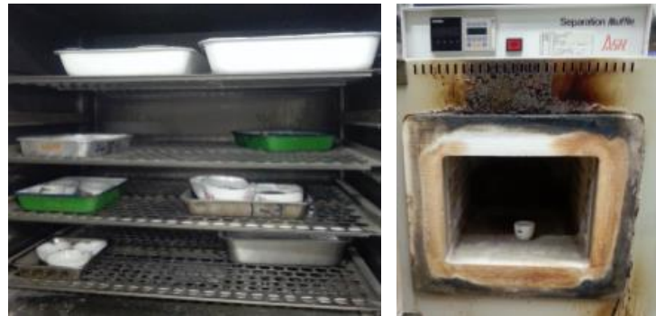
Figure 2.10: Oven and muffle furnace for moisture and ash contents test
