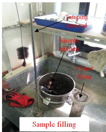
Figure 3.13: Samples filling and curing method
