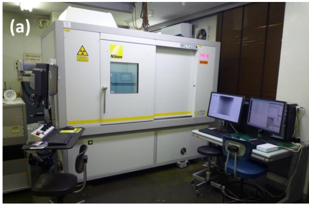
Figure 2.4: X-ray CT system, MCT225K (Nikon Instech Co.) owned by Fukuoka Industrial Technology Center. (a) MCT225K and PC for reconstructing CT images and analyzing data. (b) X-ray tube and the sample, which is fixed on the table. (c) The detector of transmission X-ray.
