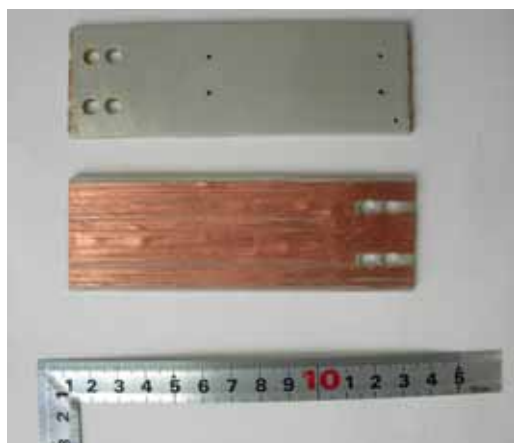
Fig.3 AlN ceramic plate with copper wire attached to one side.
