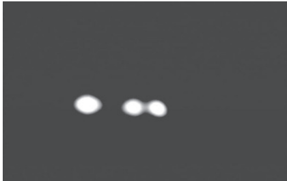
Fig. 9 Near-field-pattern of the fabricated novel active-MMI BLDs.
