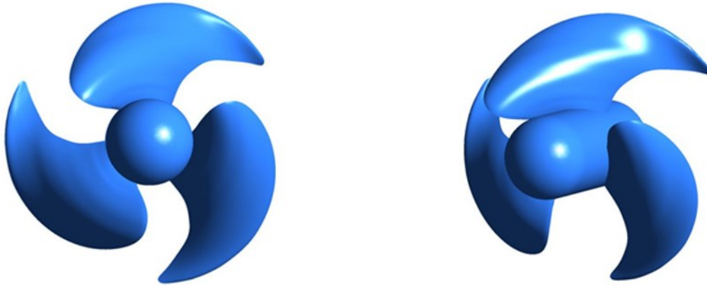
Fig. 2.6 Geometry of P4679 propeller for front view (left) and isometric view (right)
