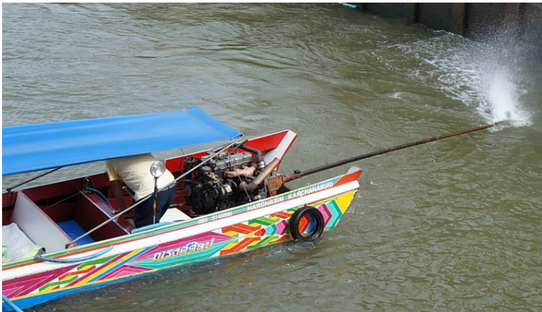
Fig. 1.6 Engine, shaft and propeller of Long-Tail Boat
