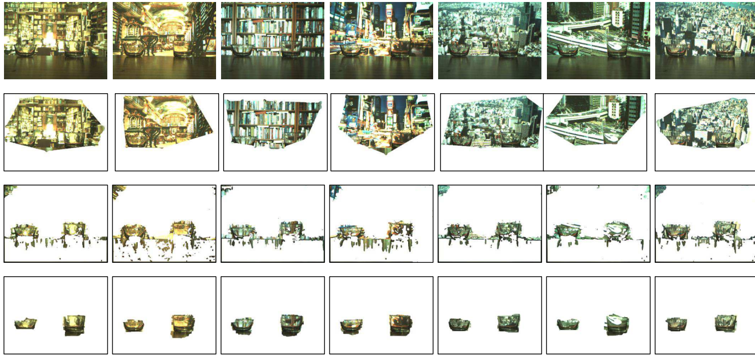
Fig. 6.8 Comparison of segmentation results for object 4 and object 5 combination in different scenes. The 1st row shows the image from the central viewpoint. The 2nd, 3rd, and 4th rows show output from the finding glass, LF-linearity thresholding, and proposed TransCut methods, respectively.
