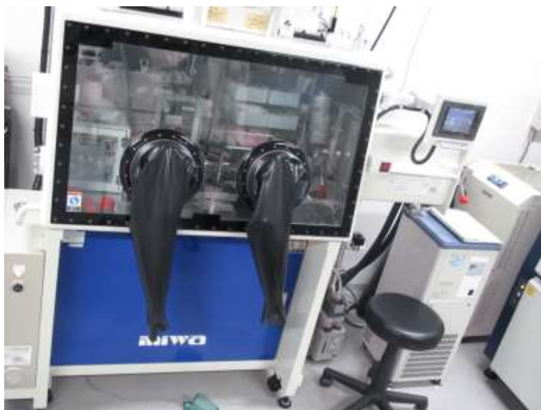
Figure 2.1 The glove box with gas purification system.
