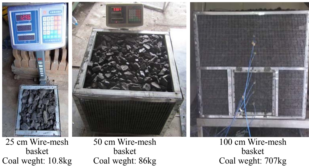
Figure 4- 3 Photos of wire-mesh basket and loaded coal in the test (Aug. 2014)
