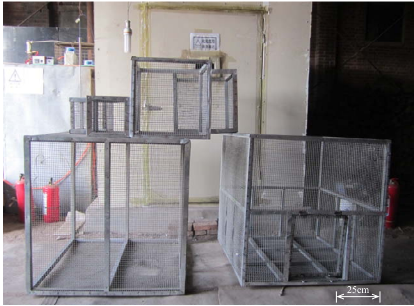
Figure 4- 2 Photo of wire-mesh baskets (25, 50, 100 cm) for upscale experiment
