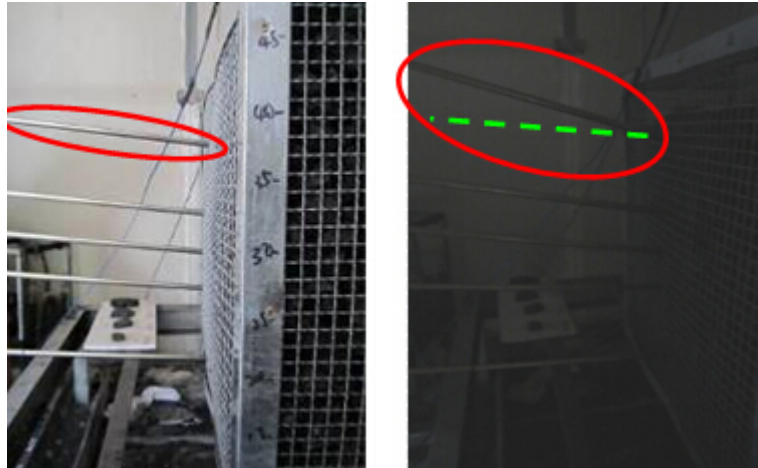
Figure 4- 16 Schematic of thermocouple position change
