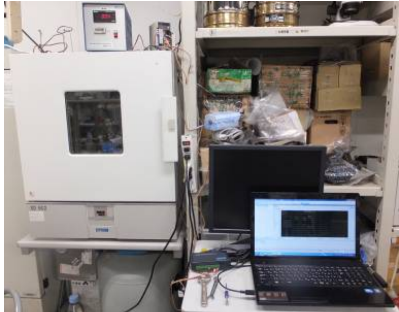
Figure 2- 3 Photo of the constant temperature system for laboratory experiment (Jan. 2013)
