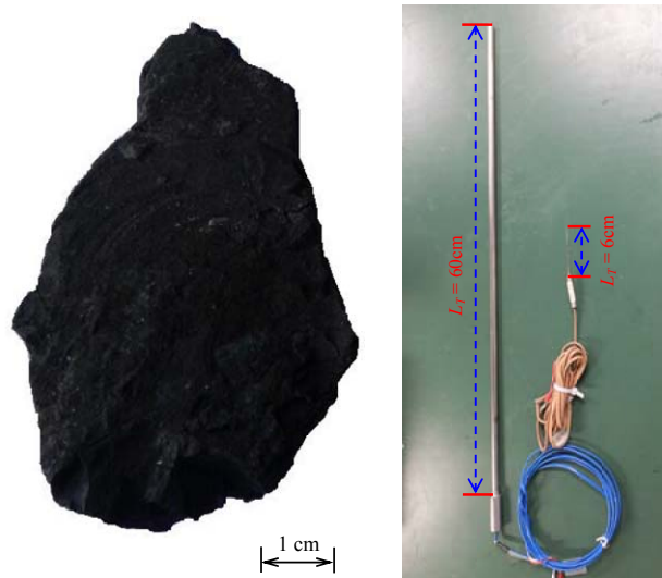
Figure 2- 13 Test coal size and thermocouple length definition Left: Typical size of the coal sample and thermocouple length; Right: L_T (unit: cm)
