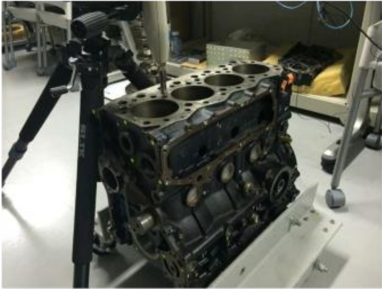
Fig.4.5 Hammer impact test to measure vibration and pressure in air
