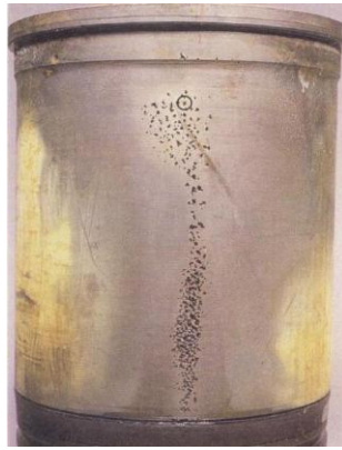
Fig.1.4 Cavitation erosion on the thrust side of real engine cylinder [25]
