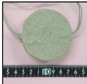
Fig 3.1 Sacrificial point anodes
