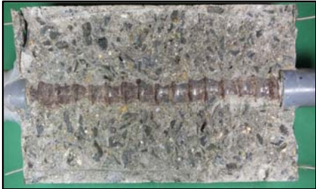
(c). Concrete with 10 kg/m 3 of chloride
