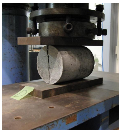
(b) Split tensile test of mortar concrete
