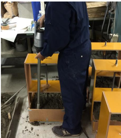
(c) Compaction process of mortar block
