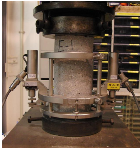
(b) Compression test of mortar concrete
