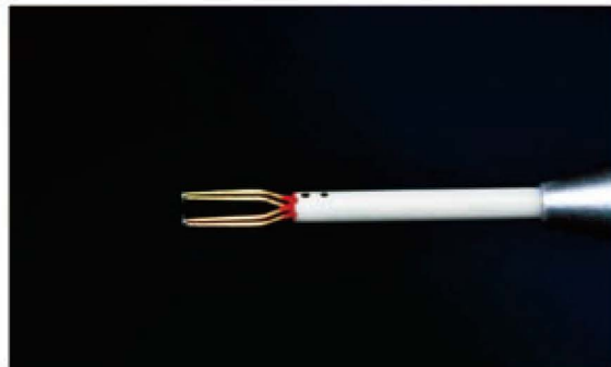
Fig. 6 Split-fiber probe, capable of detecting reversed flow
