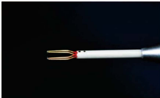
Fig. 6 Split-fiber probe, capable of detecting reversed flow
