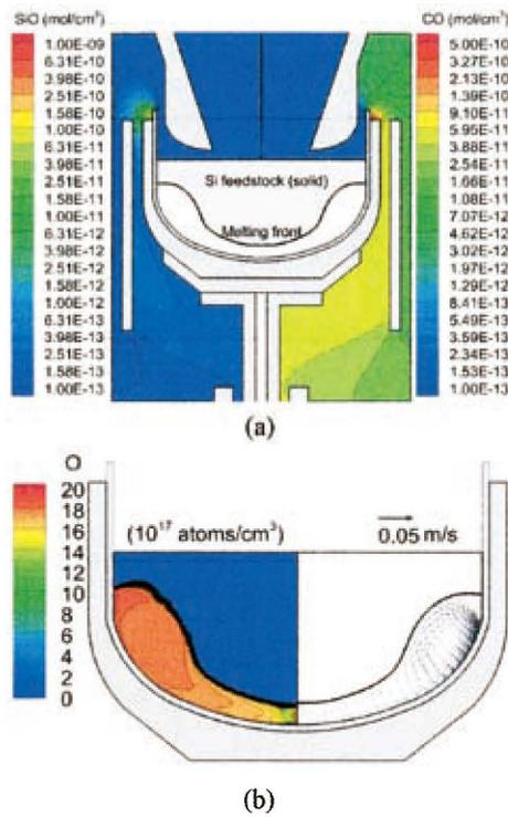
Fig. 2 Impurity transport during the first stage of the melting process: (a) Concentrations of SiO and CO in the Ar gas domain; (b) O concentration and melt flow in the Si feedstock.
