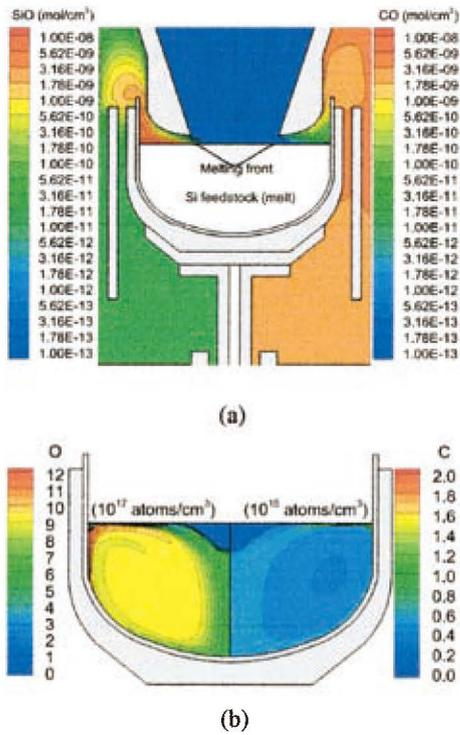
Fig. 3 Impurity transport during the second stage of the melting process: (a) Concentrations of SiO and CO in the Ar gas domain; (b) concentration of O and C in the melt.
