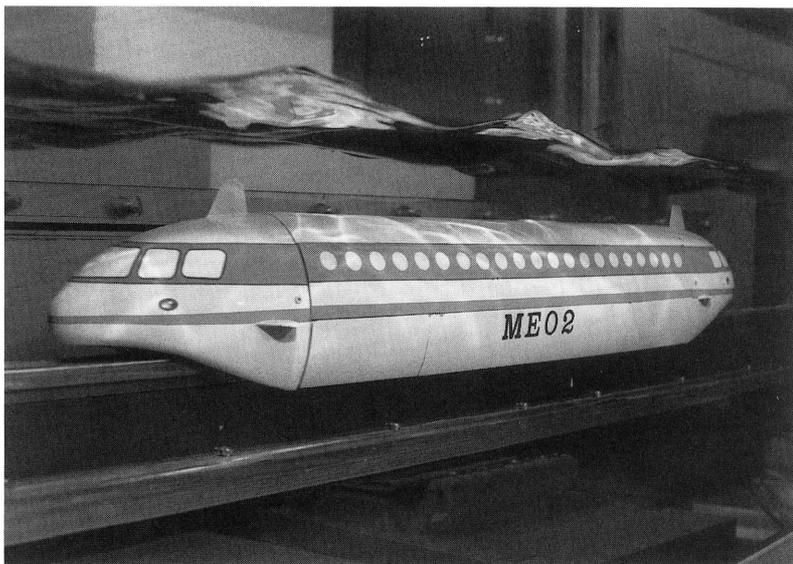
**Fig. 1** ME02 running underwater in water tank
