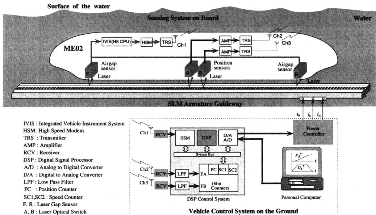
Fig. 5 Vehicle control system with no contact
