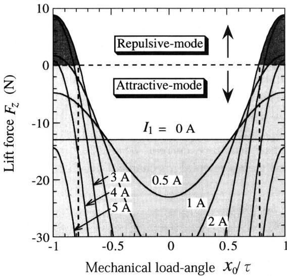
(b) Lift force vs. mechanical load-angle with a parameter of armature current
