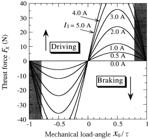
(a) Thrust force vs. mechanical load-angle with a parameter of armature current
