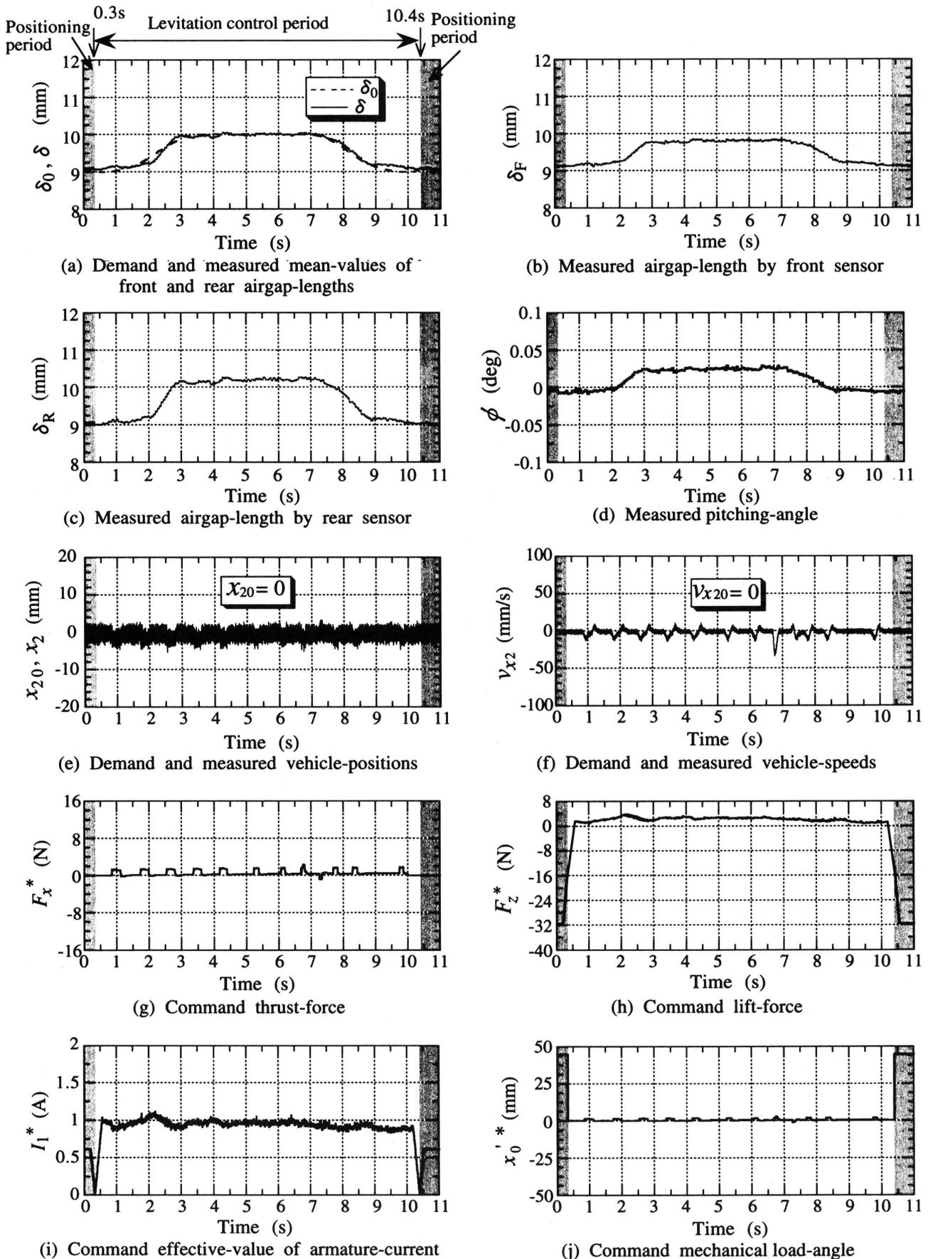
Fig. 6 Experimental results for standstill-levitation control in repulsive-mode under the water
