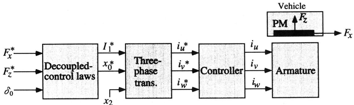
Fig. 4 Decoupled control system
