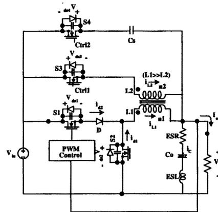
Fig.4 Complete proposed converter circuit
