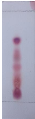
Figure A3.2. Ninhydrin staining of peptides and/or amino acid in the \leq 3 kDa fraction of ADR extract (Reishi's auto-digestion extract was spotted onto silica-gel plate (TLC Plate Silica Gel 60 F254, Merck, Darmstadt, Germany); the plate was eluted with n -butanol:acetic acid:water 3:1:1 (by volume) mixture followed by ninhydrin stain (Wako Pure Chemical, Osaka, Japan))
