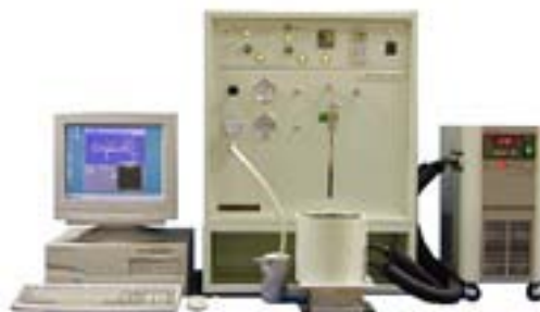
Figure 2-20. Appearance of BELSOR-HP pore analyzer instrument
