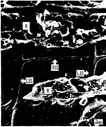
Photo. 3 Radial surface of normal wood of Hinoki, Longitudinal intercellular spaces (LIS) and a radial intercellular space (RIS) cross each other. Scanning electron micrograph.
