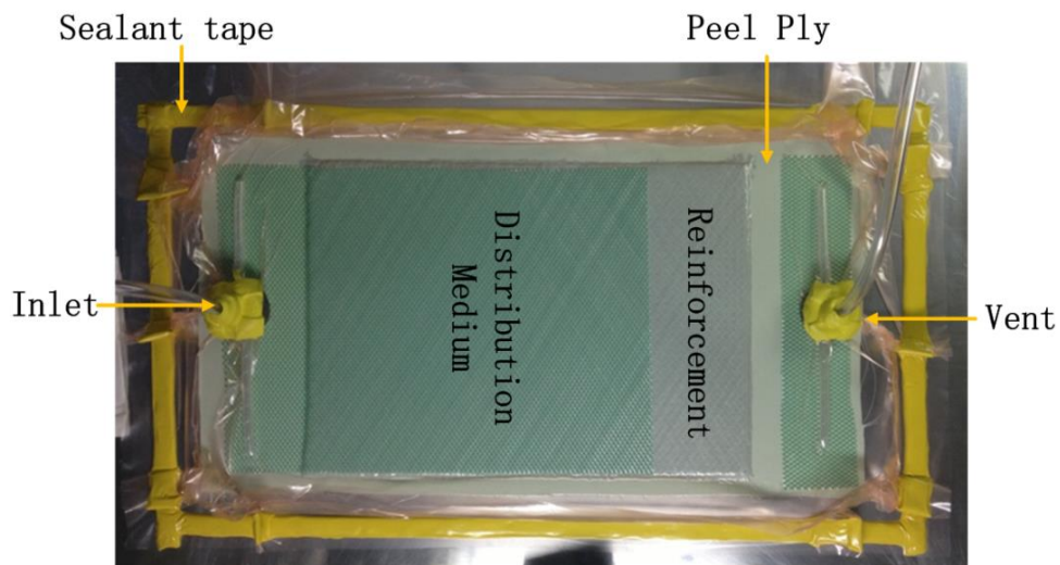
Figure 1-7 Photograph of the package in a VARTM process.
